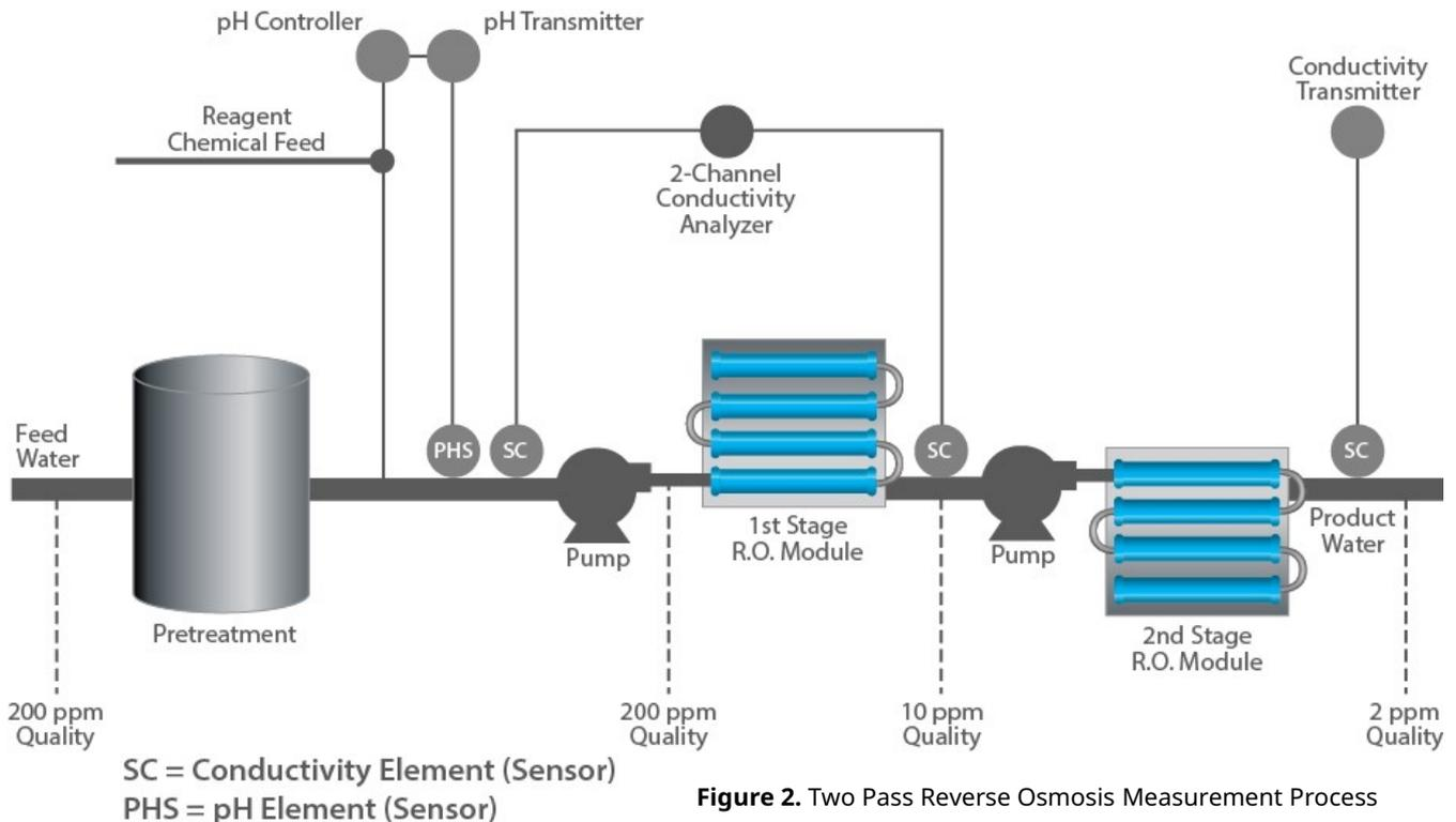
Figure 2. Two Pass Reverse Osmosis Measurement Process
