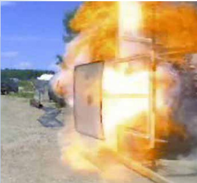
Dynamic testing of a VSB building vent
